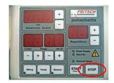
**5.** To save and end setup mode, press the STOP button.
