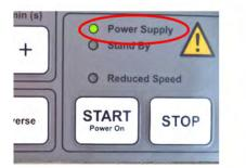
**3.** If POWER SUPPLY is flashing, the device is in setup mode. If POWER SUPPLY is not flashing, repeat the procedure.
