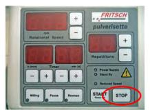
**1.** Press and hold the STOP button on the front of the control panel.
