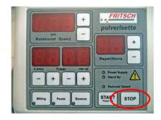
**1.** When the device has been switched off, press and hold the STOP button on the front control panel.
