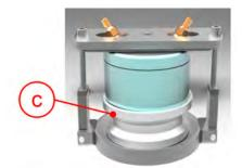
**3.** When using grinding bowls with a volume of 80 ml, the adapter piece (90.1120.09) has to be used as well.
