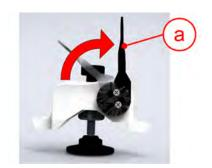
2. Hang the longer projection of the Safe-Lock tensioning device into one side of the mounting of the grinding bowl holder.
