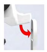
**3.** Hang the short projection of the Safe-Lock tensioning device into the other side.
