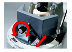
The counterweight (6) has to be positioned according to the scale in order to offset the imbalance and thus prevent the mill from shifting.
