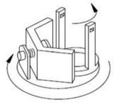
The grinding stock is crushed and ground by grinding balls in a grinding bowl. The centrifugal forces resulting from the rotation of the grinding bowls around their own axes and from the rotating support disc (14) influence the contents of the grinding bowl consisting of grinding stock and grinding balls.
