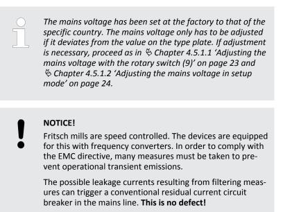
To prevent this, special residual current circuit breakers, which are adapted for operation with frequency converters, are commercially available.
