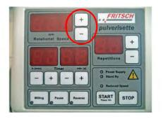
**4.** Use the +/- ROTATIONAL SPEED buttons to adjust the level of the mains voltage (90-260 V) to the existing mains system.
