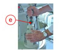
**5.** Pre-tension the setting screw (b) manually, then place the provided torque spanner on the setting screw (b) and turn until it clicks.
